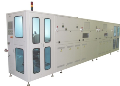
Tape casting on polyester film
